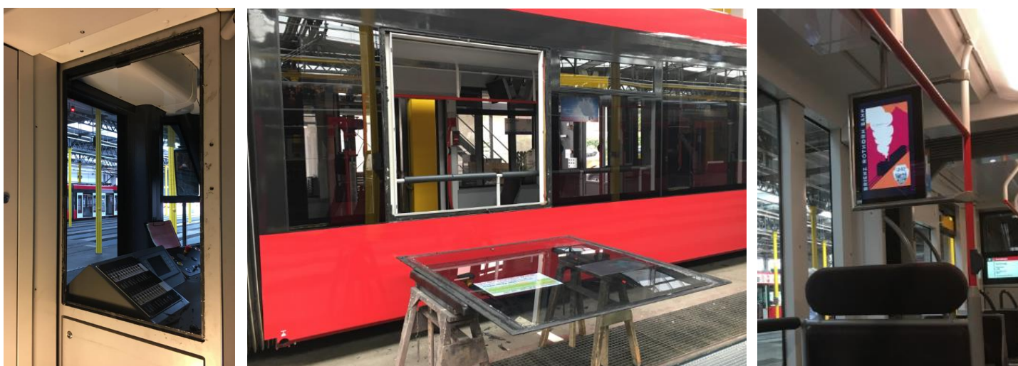
Assembly process of the side-window and partitions systems in the Combino XL tram car
