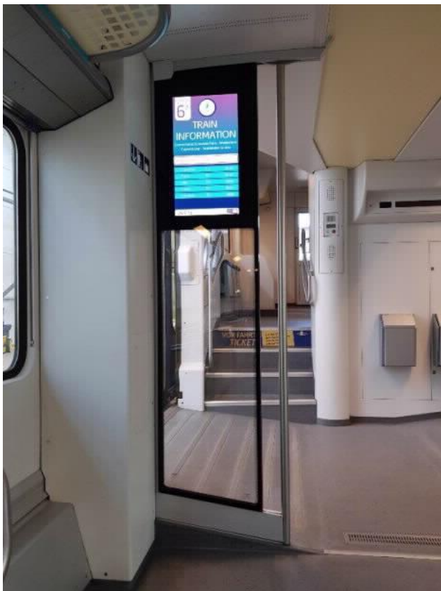
ScreeneX TRN 21-2 in Full IGU configuration; the surrounding silk-print is designed to conceal the sealing element of the IGU
