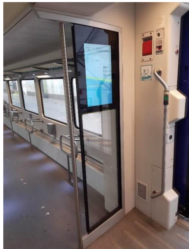
ScreeneX TRN 21-2 in Full IGU configuration; the surrounding silk-print is designed to conceal the sealing element of the IGU
